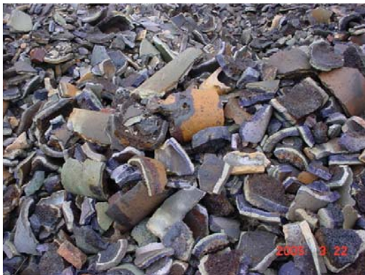
Broken retorts at the East La Harpe smelter. The extreme heat and minerals of the distilling furnaces cause the multiple colors on the surface of the retorts.
