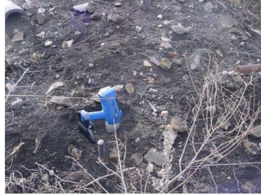
An XRF analyzer used for field screening.
