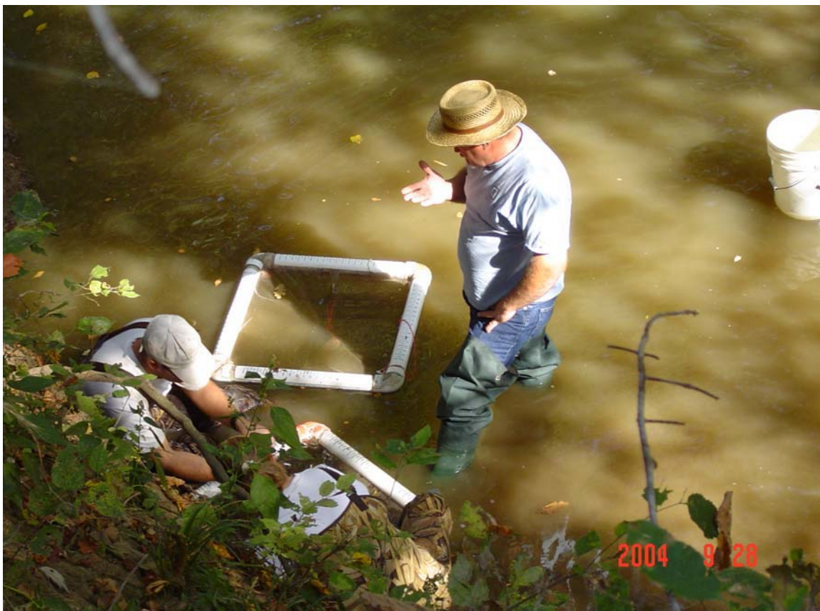
Fish and sediment sampling downstream of the Cherryvale smelter in order to identify the impact of contamination on surface waters.
